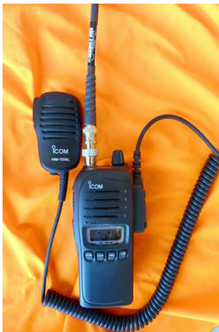
The IC-41s with high gain antenna and speaker/microphone kit.
